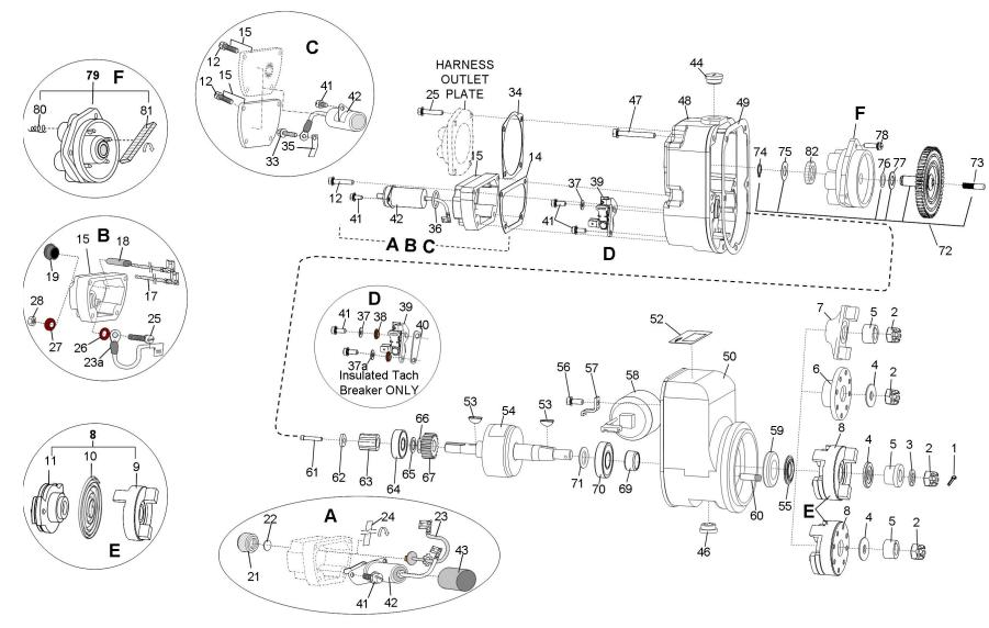
Figure 1. S-20/S-200 Series Magneto - Exploded View
